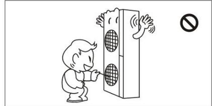
Do not touch the air outlet grill when fan motor is running.
