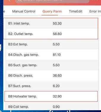
• If no air in the pipeline after checking, and the temperature difference exceeds 10 degrees after the water flow switch is short-circuited, it is necessary to replace the pump with a larger head and flow rate
